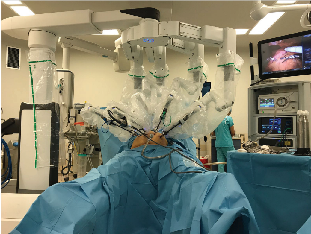
Figure 2. Intraoperative photo showing the position of the Xi robot after docking.
